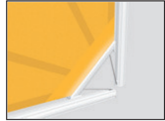
Guide tracks with extremely high tensile strength tensioning cords
